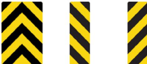
Figure 6. Balises de danger D-290, D-290-D et D-290-G
